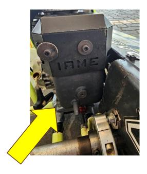
This is strictly limited to the **lower half—no other portions** of the shield or engine components may be modified.
